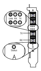
Figure 3. Location of the LEDs (dual link)
